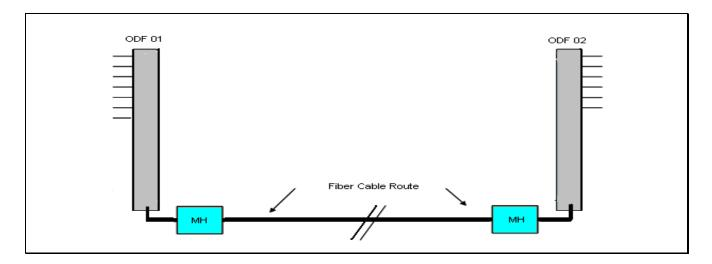
Figure 9: Connection between Aggregate Point to Aggregate Point - Ring Network
