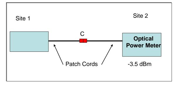
Laser Source Verification Procedure with Simple Signal Insertion and Detection Tester
