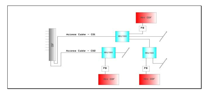
Figure 8: Connection between Aggregate Point to the Entities - Access Network
