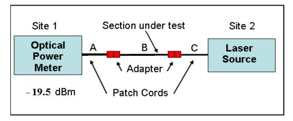
**NOTE:** Each reading must be performed in both directions. The result is divided by two (2) to obtain the real value.
