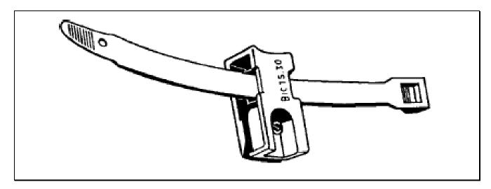
Aerial Cable Mount (for Steel, Concrete, and Wooden Poles)
